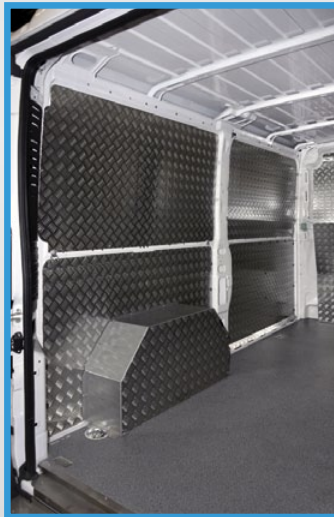
Ducato/Boxer/Jumper 2006: marble-look panel floor, Complete panelling in checkered aluminium, Bulkhead cover in checkered aluminium, Wheel cover in aluminium/steel
