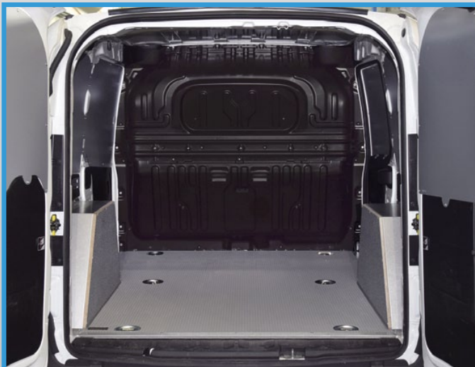
Doblò 2010/Combo 2012: Wooden flooring rubberized, Wheel cover plywood resin finish marble colour/steel, side lining in painted metal sheet
