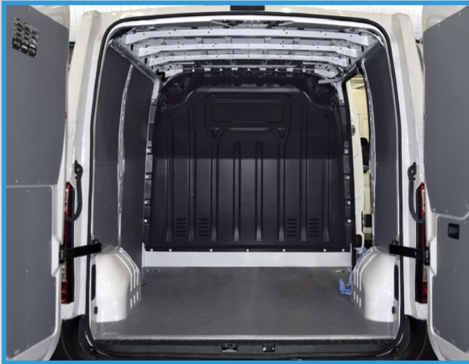
Master/Movano/NV400 2010: marble-look panel floor, side lining in painted metal sheet
