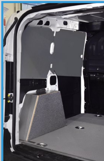
Doblò 2010/Combo 2012: Wooden flooring rubberized, Wheel cover plywood resin finish marble colour/steel, side lining in painted metal sheet
