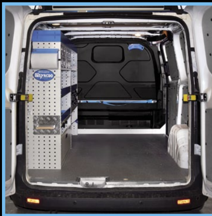
Ford Custom: racking installation on the left side.
