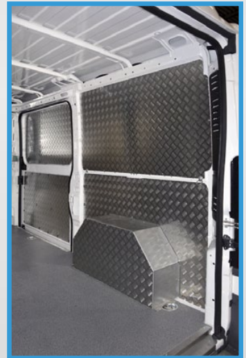
Ducato/Boxer/Jumper 2006: marble-look panel floor, Complete panelling in checkered aluminium, Bulkhead cover in checkered aluminium, Wheel cover in aluminium/steel
