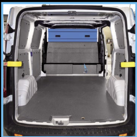
Ford Custom: wall-mounted racking leaves the entire floor free for cargo.
