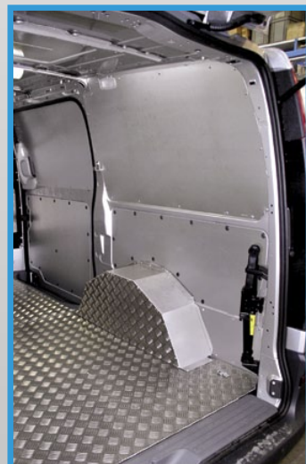
Vito 2004: Checkered aluminium flooring, complete panelling in aluminium, wheel cover in aluminium/steel, bulkhead cover in checkered aluminium
