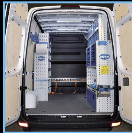
Mercedes Sprinter: racking along part of both side walls.
