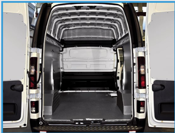
Vivaro/Trafic 2014/Talento 2016/NV300 H1: marble-look panel floor, side lining in painted metal sheet, wheel cover in aluminium/steel
