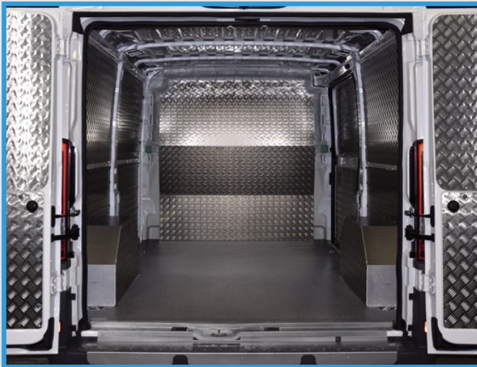
Ducato/Boxer/Jumper 2006: marble-look panel floor, Complete panelling in checkered aluminium, Bulkhead cover in checkered aluminium, Wheel cover in aluminium/steel
