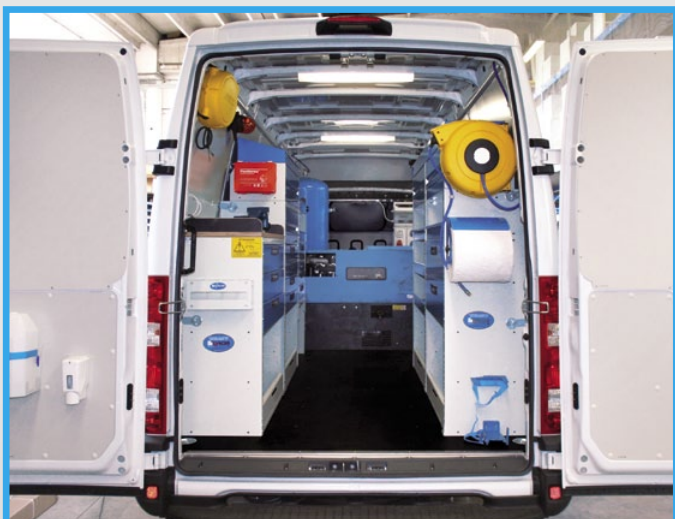
Iveco Daily with storage shelves, provided with 15 KVA generator and compressor.
