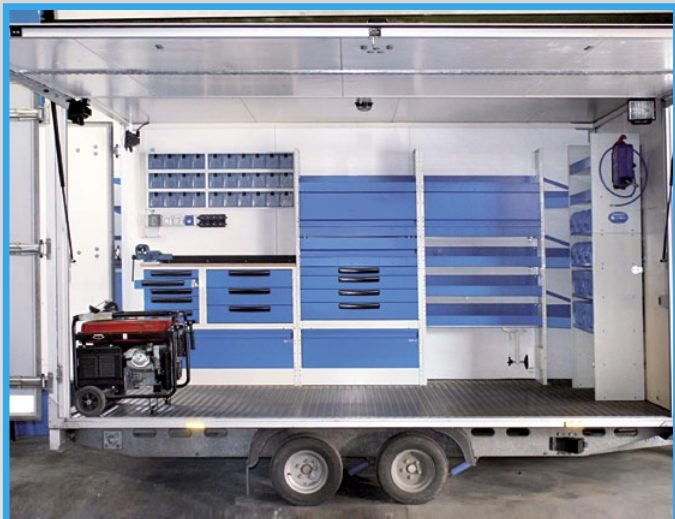
Mobile workshop inside a trailer in aluminium and fibreglass.
