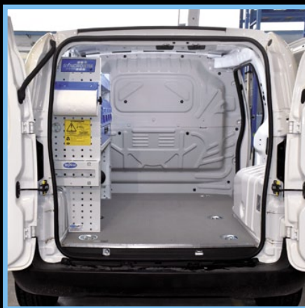
Fiat Fiorino: racking installation on the left side.
