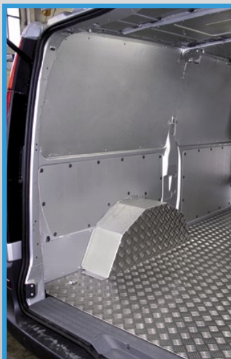
Vito 2004: Checkered aluminium flooring, complete panelling in aluminium, wheel cover in aluminium/steel, bulkhead cover in checkered aluminium
