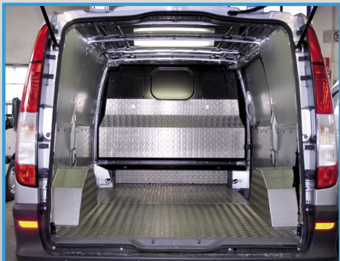
Vito 2004: Checkered aluminium flooring, complete panelling in aluminium, wheel cover in aluminium/steel, bulkhead cover in checkered aluminium
